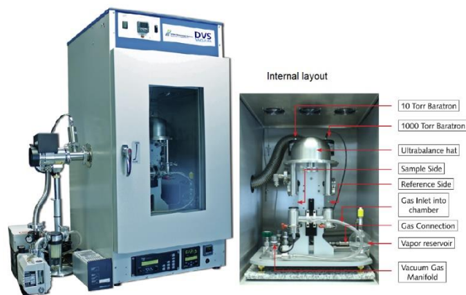
Figure 4 – DVS Vacuum gravimetric sorption analyzer [14]
